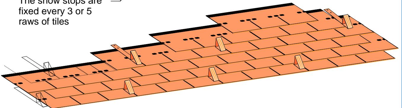
The drawing shows the position of snow stops every 3 rows of tiles, to obtain a density of snow stops of 2,33 pieces every m<sup>2</sup> (25 sq.).
